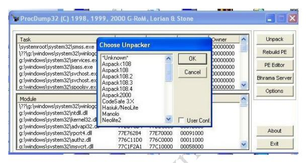
5) **File Analyzers**: - To identify which packer is used to pack file cracker uses this kind of programs. By using this, a cracker can know which compiler or packer is used to protect the shareware. This software simply works on signature byte. With the help of this you can find what compiler or in which language the program has written. There are many this kind of program are available such as file inspector, File Info etc.
